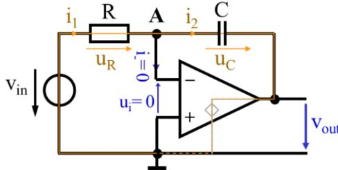
$$u_i = 0 \Rightarrow u_R = v_{in} \Rightarrow i_1 = \frac{v_{in}}{R}$$
