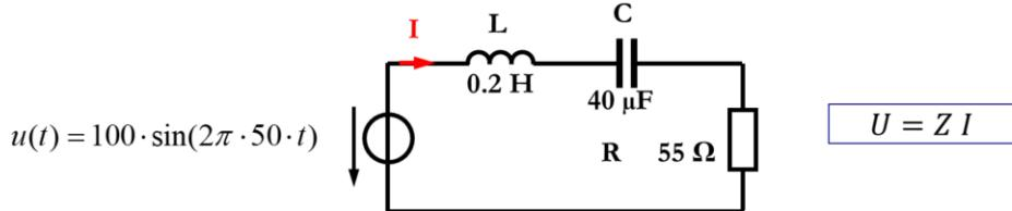
$$Z = R + j\omega L + \frac{1}{j\omega C} = R + j(\omega L - \frac{1}{\omega C}) = 55 + j(63 - 80) = 55 - j17 \text{ } (\Omega)$$
