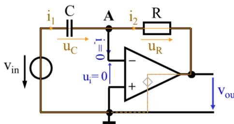
$$u_i = 0 \Rightarrow u_C = v_{in} \Rightarrow i_1 = C \frac{dv_{in}}{dt}$$
