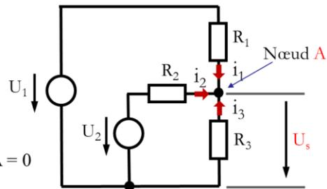
$$\frac{U_1 - U_s}{R_1} + \frac{U_2 - U_s}{R_2} + \frac{-U_s}{R_3} = 0 \quad \Rightarrow$$
