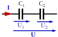
$$U = U_1 + U_2 = \frac{1}{C_1} \int I dt + \frac{1}{C_2} \int I dt = \left( \frac{1}{C_1} + \frac{1}{C_2} \right) \int I dt = \frac{1}{C_{eq}} \int I dt$$
