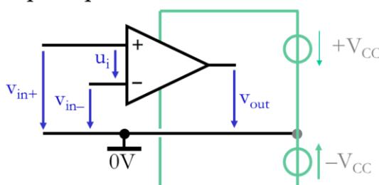
$$v_{out} = A \cdot (v_{in+} - v_{in-}) = A \cdot u_i$$
