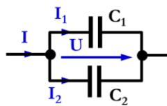
$$I = I_1 + I_2 = C_1 \frac{dU}{dt} + C_2 \frac{dU}{dt} = (C_1 + C_2) \frac{dU}{dt} = C_{eq} \frac{dU}{dt}$$
