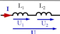
$$U = U_1 + U_2 = L_1 \frac{dI}{dt} + L_2 \frac{dI}{dt} = (L_1 + L_2) \frac{dI}{dt} = L_{eq} \frac{dI}{dt}$$
