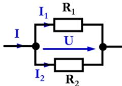
$$I = I_1 + I_2 = \frac{U}{R_1} + \frac{U}{R_2} = \left(\frac{1}{R_1} + \frac{1}{R_2}\right)U = \frac{1}{R_{eq}}U$$
