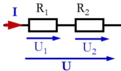
$$U = U_1 + U_2 = R_1 I + R_2 I = (R_1 + R_2) I = R_{eq} I$$
